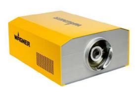
The patented technology of the Layer Check LC 1000 is based on thermal optics and enables seamless logging during the coating process by means of constant measurement. Non-contact and non-destructive layer thickness measurement is carried out at a distance of up to 50 cm from the workpiece. Overcoatings are prevented, resulting in material savings of up to 30% for powder and corresponding cost savings. Undercoating with too little
